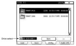
When using Drive Select to select a hard disk, the ID numbers of hard disks that have not been formatted will appear as Unformatted, and the ID numbers of hard disks that are not connected will appear as None. Even if a hard disk has been formatted by a personal computer, etc., it will be shown as Unformatted, and such a hard disk must be formatted as well.
